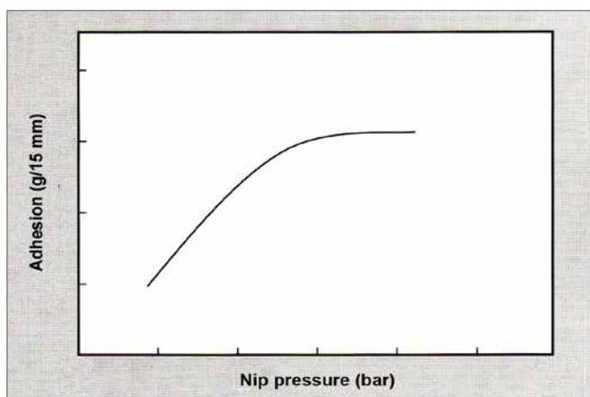
**Figure 11:** Effect of Nip Pressure on Adhesion of Extrusion-Coated LDPE to Porous and Non-Porous Substrates
