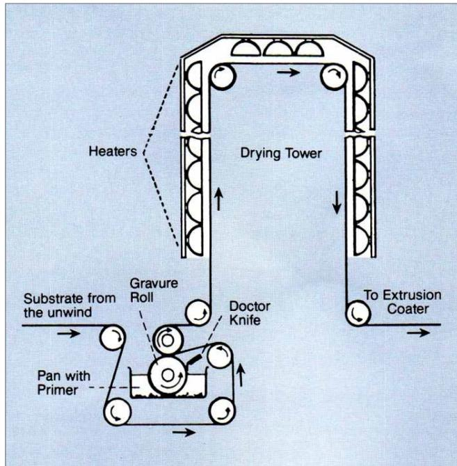
**Figure 14:** Schematic Drawing of Typical Priming Station
