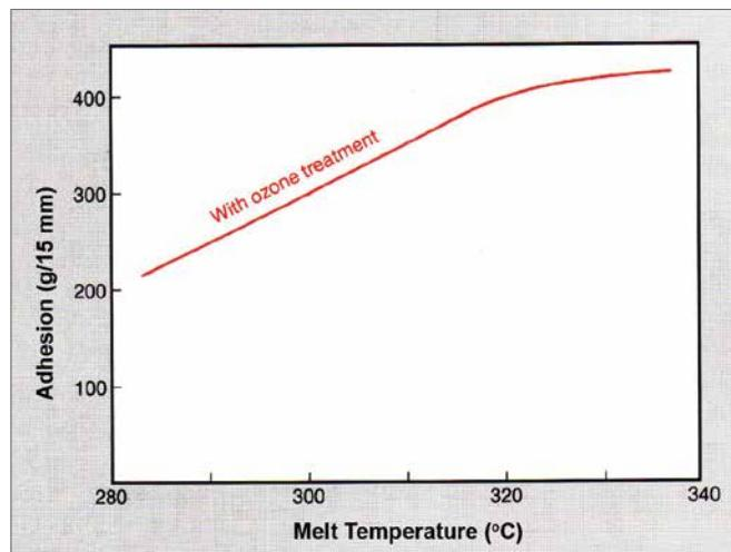
**Figure 9: Effect of Melt Temperature and Ozone Treatment on Adhesion of Extrusion-Coated LDPE to Aluminium Foil**
