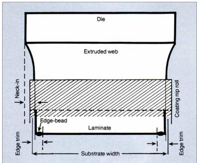
**Figure 4:** “Neck-in” During Extrusion Coating
