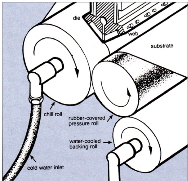
**Figure 3: Typical Extrusion Coating Nip Roll Assembly**
