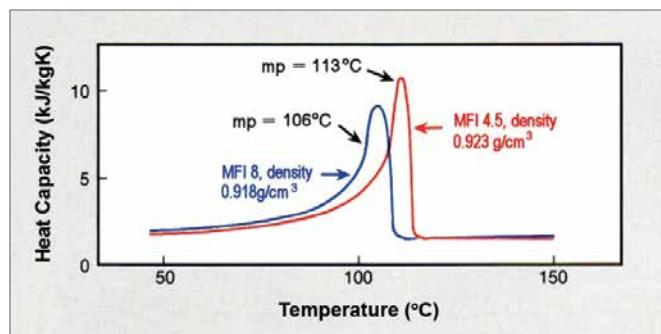
**Figure 15:** Melting Point and Heat of Fusion for Alkathene LDPE Extrusion Coating Polymers. (Determined by Differential Scanning Calorimetry)
