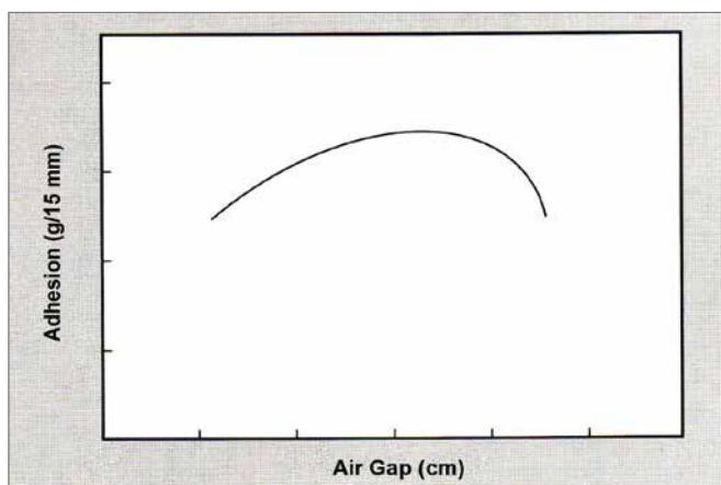
**Figure 12:** Effect of Air Gap on Adhesion of Extrusion-Coated LDPE to Non-Porous Substrates
