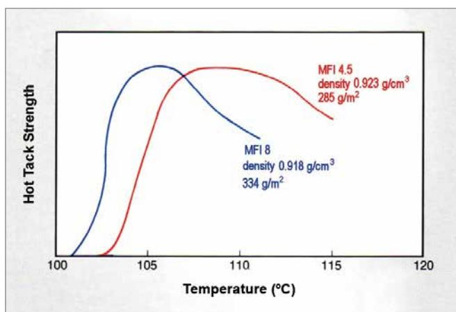
**Figure 17:** Typical Hot Tack Strength Characteristics of Alkathene LDPE Extrusion Coating Polymers.
